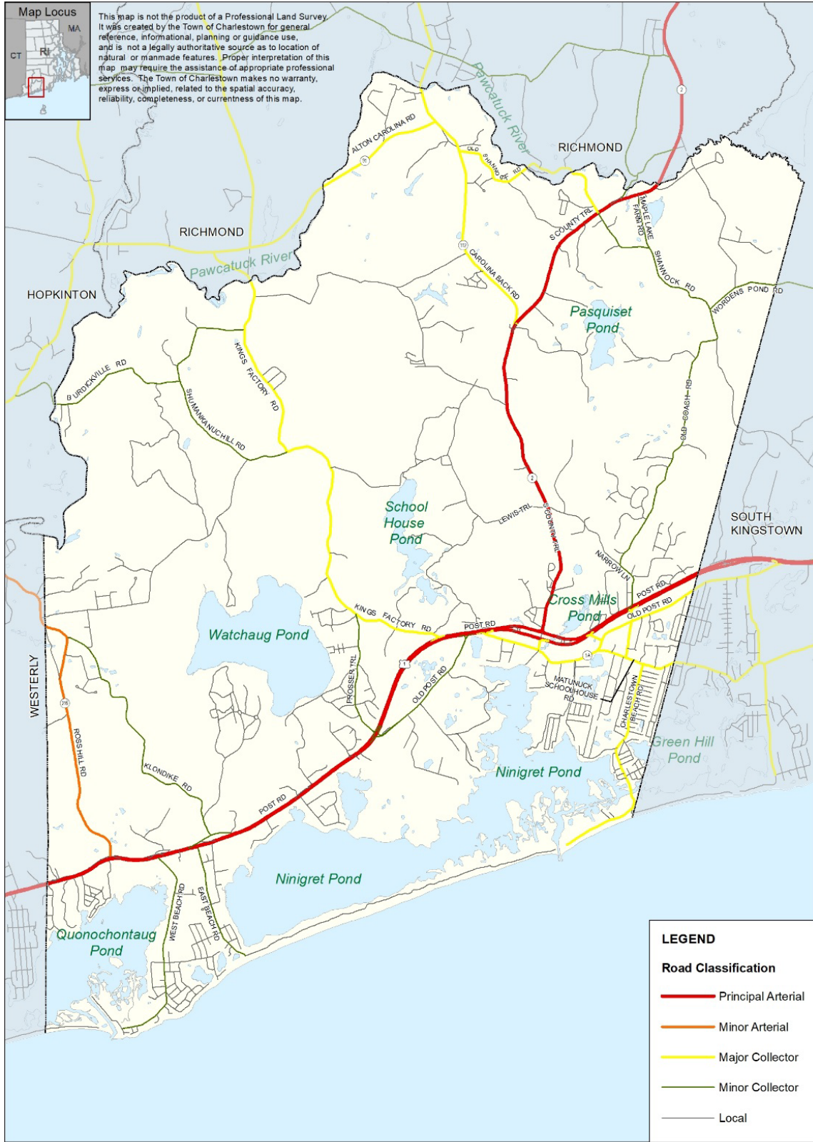
Figure TR-1 Highway Functional Classifications of Roads in Charlestown Source: Statewide Planning Program, RI DOT, RI GIS
