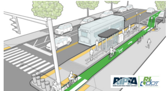
Graphic showing the design of bike lane bypass around a bus stop from the RIPTA Bus Stop Design Guide, courtesy of RIPTA
