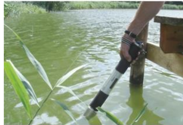
Algae torch: In-situ sensor for blue-green algae levels in seconds
