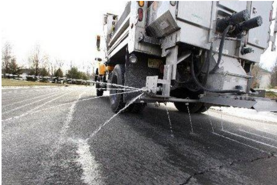
(Brine (saltwater) being applied to road surface, Jerry McCrea/The Star-Ledger)
