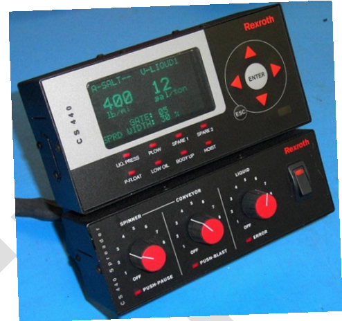
Closed-loop Snowplow Control Module used by RIDOT, Photo: mto.gov.on.ca)
