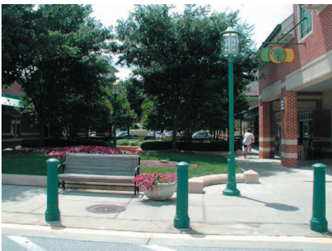
Pedestrian lighting directs light on sidewalk and bench and bollards create a barrier between pedestrians and traffic
